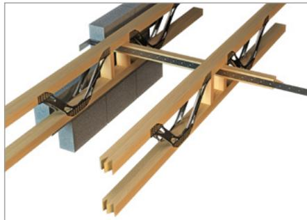
Perpendicular lateral restraint
