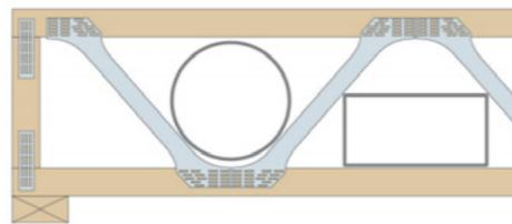
All joists are designed to accommodate a minimum 100mm nominal round soil and vent pipe SVP or rectangular 50mm x 300mm section ducting.
