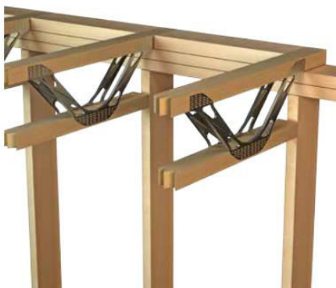
TF3 - Top Chord Support on Over-height Panel - External Wall
